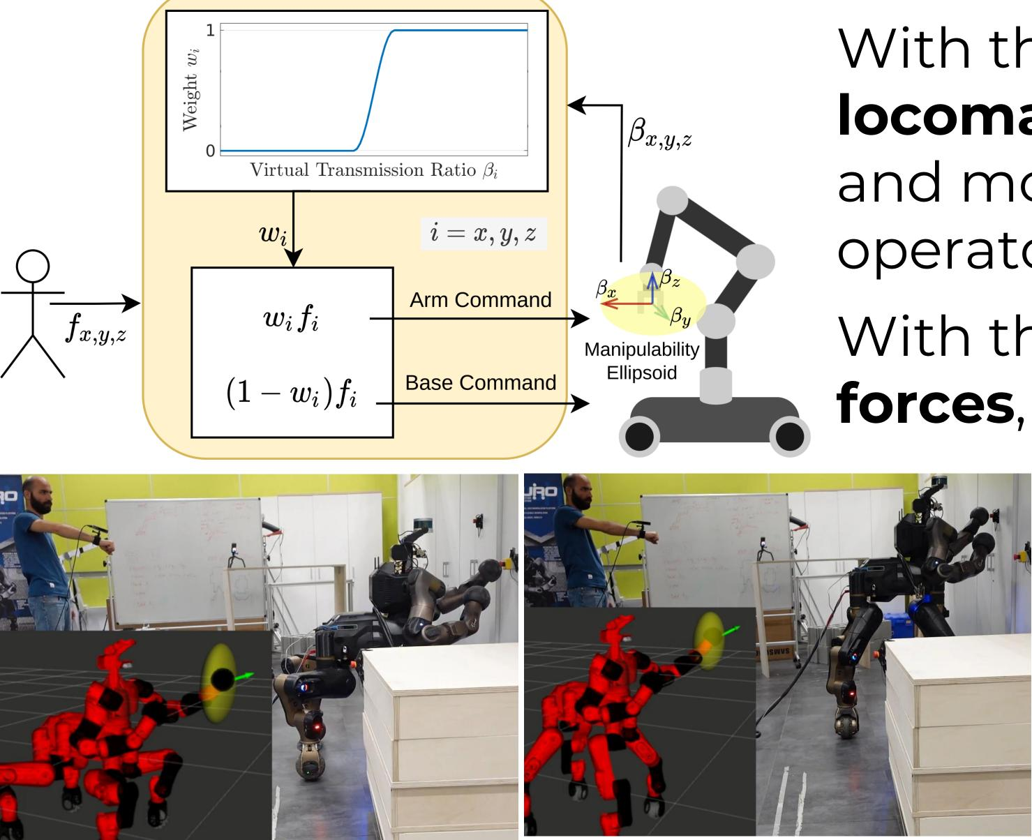
With the manipulability-aware shared locomanipulation, the interface generates arm and mobile base commands from a single operator input
