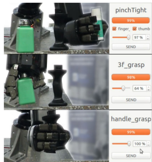
Fig. 14 The three grasping actions performed during the experiment with HERI II hand and IIT-INAIL arm. On the right side, the GUI shows the grasping actions in execution. The loading bars are not fully completed (to 100%) because of small errors in tracking the actuator reference positions
