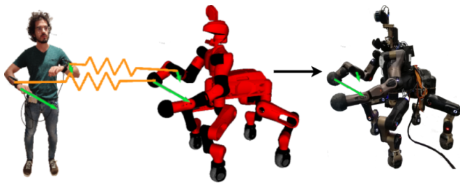
Fig. 2. The TelePhysicalOperation concept follows a “Marionette” type interaction: the operator generates virtual forces that can be selectively applied on specific locations on the robot segments.
